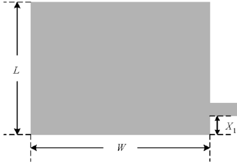
Figure 2, Dimension of the one of the four microstrip patch. W=8\text{mm} , L=6\text{mm} , X1=0.4\text{mm} .
